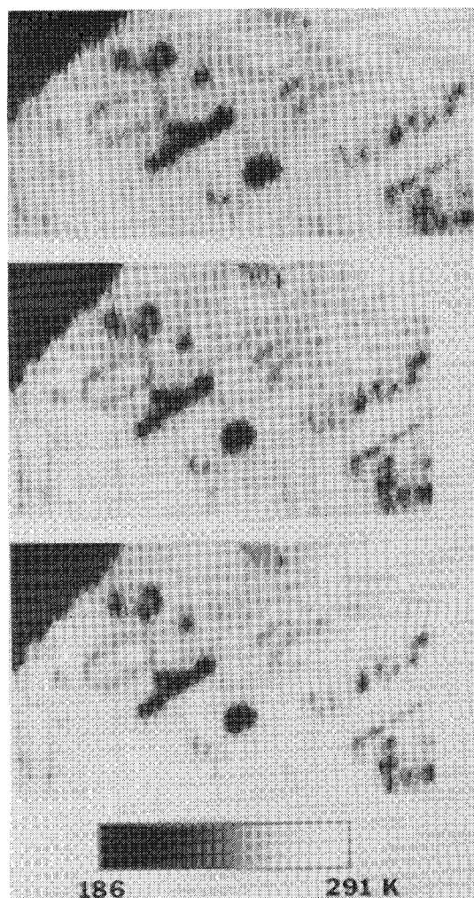
Fig. 3. An example of data processing using a portion of the imagery from the fourth row of Fig. 2. The unprocessed image is at the top; the processed image is shown in the middle. The bottom image shows the result of removing the sharp edges produced by quantizing the image into resolution elements. This improves pattern recognition and ease of viewing without the sacrifice of any significant spatial resolution. The antenna temperature of all three images is given by the grey scale at the bottom.
